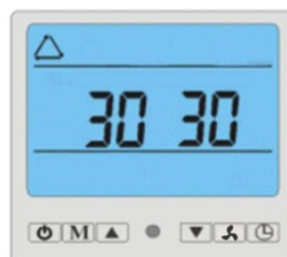
Picture: Parameters check, input water temperature 30°C.
