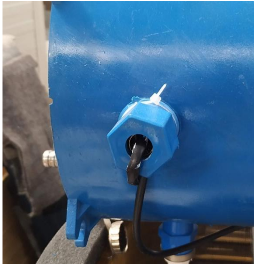
T4 – Compressor discharge temperature
