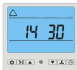
Picture: Parameters check, input water temperature 30°C.
