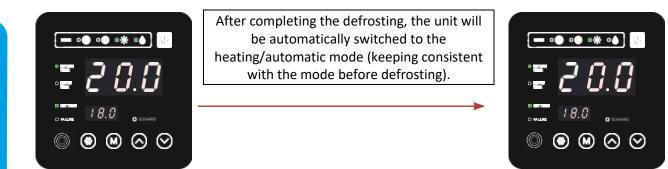
Notes: During the defrosting, mode switch is available. And when switching the mode, the unit won't work under a new mode until defrosting is completed.
