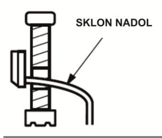
Proper installation of condensate hose
