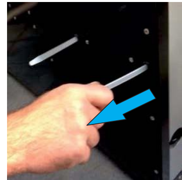
Img. 3: Finally, pull the tape out of the device and remove it.
