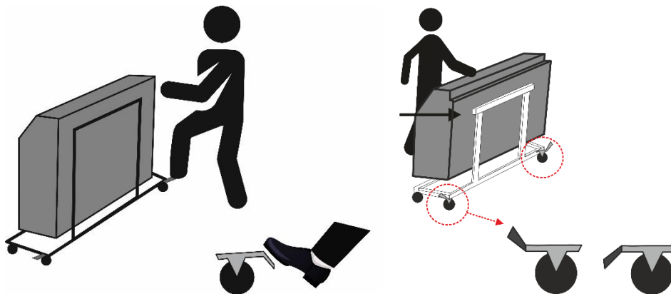
Obr.1 After moving Athmoss on the mobile stand to the application site, secure the wheel brake (locking). The wheel brake is locked when the brake lever is down. The wheel brake is released when the lever is up.
