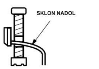
Proper installation of condensate hose
