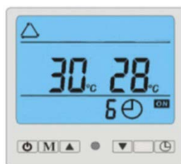
Picture: Timer set on. Heat pump to start in 6 hours.
