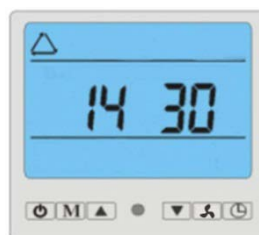
Picture: Parameters check, input water temperature 30°C.
